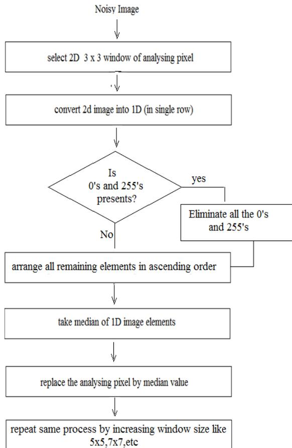
Fig 4. structure of Decision Based Adaptive Median filter
