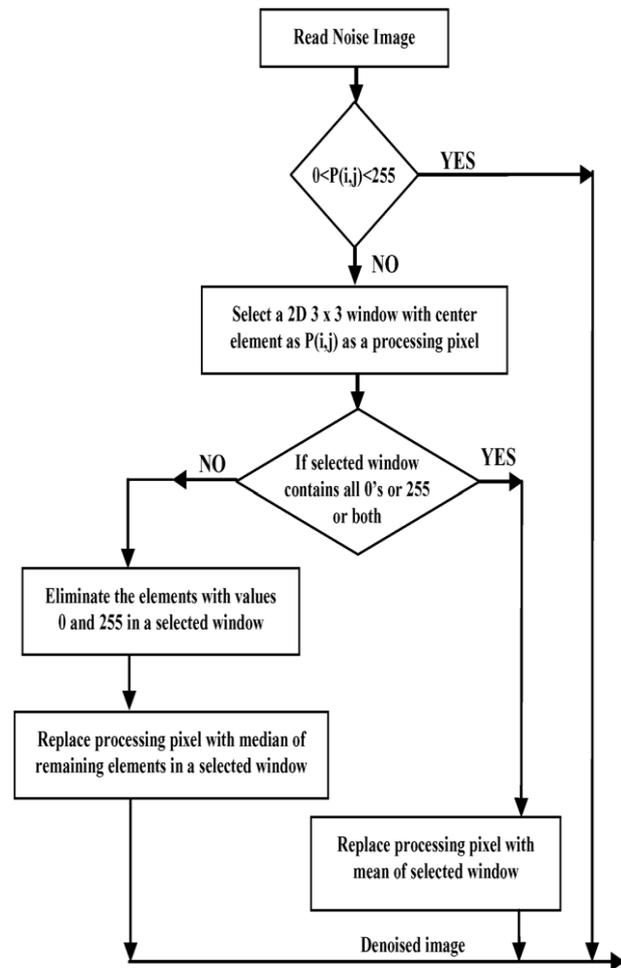
Fig 5. Structure of modified Decision Based Unsymmetric Trimmed Median filter
